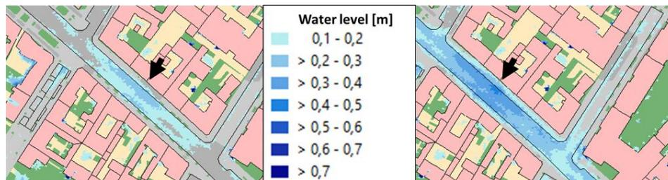
**Figure 3.** Maximum water levels in the centre of flooding due to R1. Left: heterogeneous distribution of retention roofs (implementation approach 1); right: homogeneous distribution of retention roofs (implementation approach 2), each with a degree of implementation of approx. 50 %.
