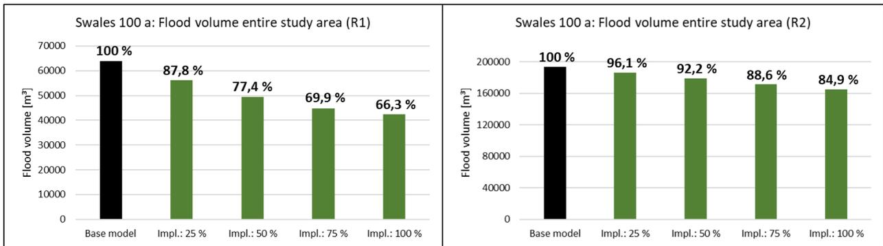
**Figure 1.** Total flood volume without BGI (base model) and with different degrees of implementation of swales (sized to T = 100 a). The figure on the left shows the total flood volume for R1, the figure on the right for R2
